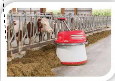
Automated Feeding System
